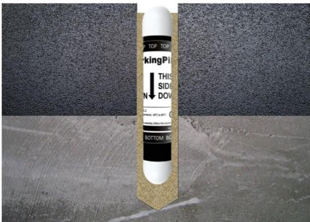
**Figure 4:** Hole filled with sand.
